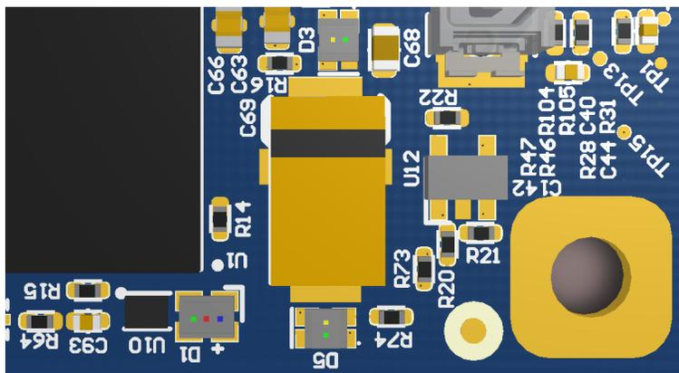
Figure 2: Combined LED Arrangement
